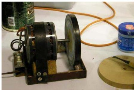
Joe brought in a small motor fitted with an 8" diameter wooden wheel he made himself. The wheel was simply made from MDF (medium-density fiberboard). You could also purchase a wheel that is basically the same for about \$20.
